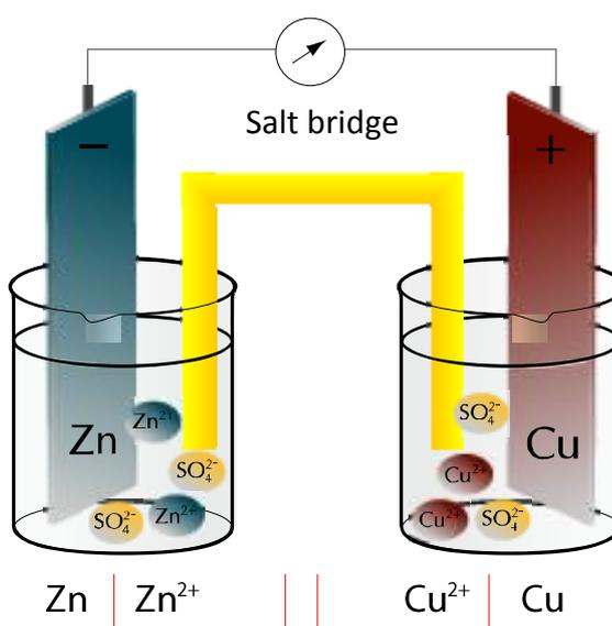
The electric potential of a cell is defined as the difference of the potentials between the electrodes of inoperative cell:
